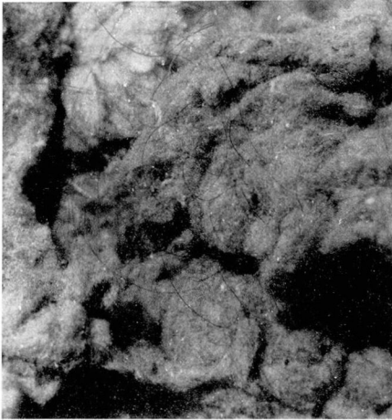
Fig. 9. Close view of debris showing admixture of human hair in the cotton debris worn off the inside of the gowns and wearers' underwear.
