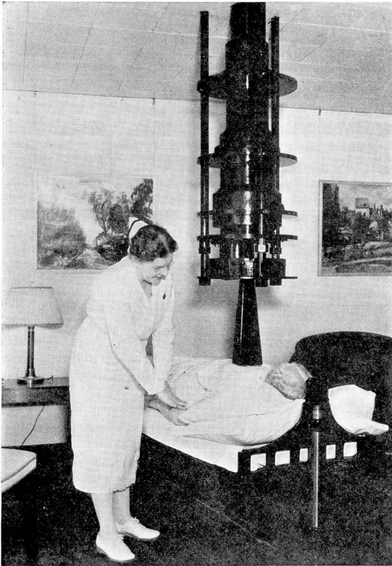
FIGURE 5: Lower end of 1200 KV roentgen ray tube (see fig. 4) in treatment room.
