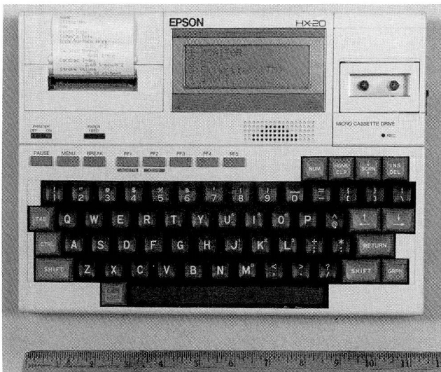
Fig. 1. Epson HX-20 programmable computer with built-in printer and cassette drive.
