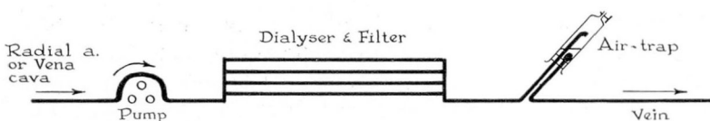
FIG. 3. Blood is forced into the apparatus either by arterial blood pressure or by a pump or both. The blood in the apparatus is under pressure varying from 260 to 20 mm. Hg. In addition, suction may be applied to the rinsing fluid which increases the filtration pressure.
