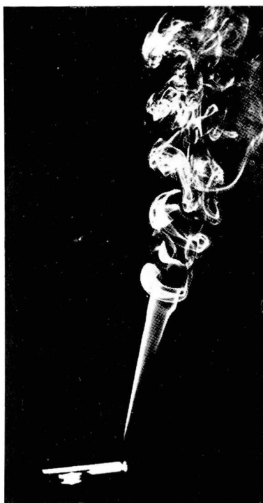
Fig. 1. The difference between laminar and turbulent flows can be seen by watching the smoke rising from a cigarette in a still room.
