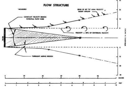
Fig. 4. Demonstration of measured air patterns.
