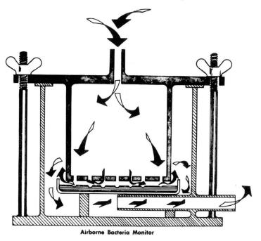
Fig. 8. New type air sampler.
