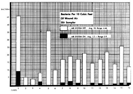
Fig. 10. Slit sampler, bacterial count.
