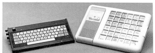
Fig. 2. Synthesized speech devices. The Say-It-All (left) provides limitless speech capacity with a memory component for 128 phrases. The Vocaid (right) provides preselected, common phrases.
