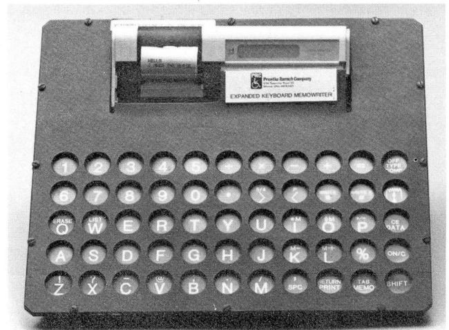
Fig. 1. The Expanded Keyboard Memowriter functions as a minitypewriter with limited memory capacity.
